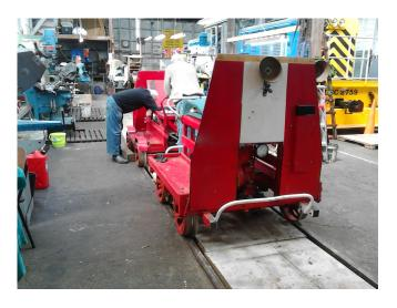
During the weekend it was found to be rather hard to get the engine started and various amounts of black and white smoke were observed coming out of the exhaust. It has been returned to the company which fitted the replacement engine to have more work done on it
